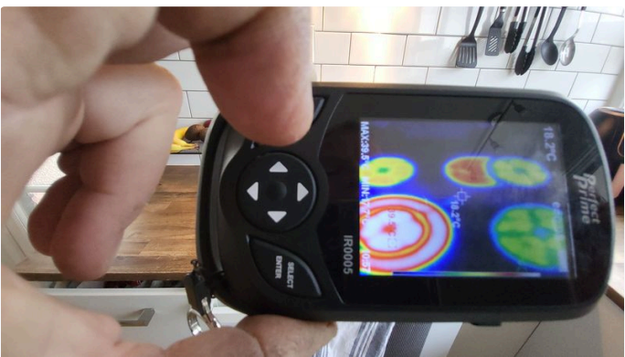
Ref #17.6 - Electric elements Observed Functioning at the time of the inspection;
