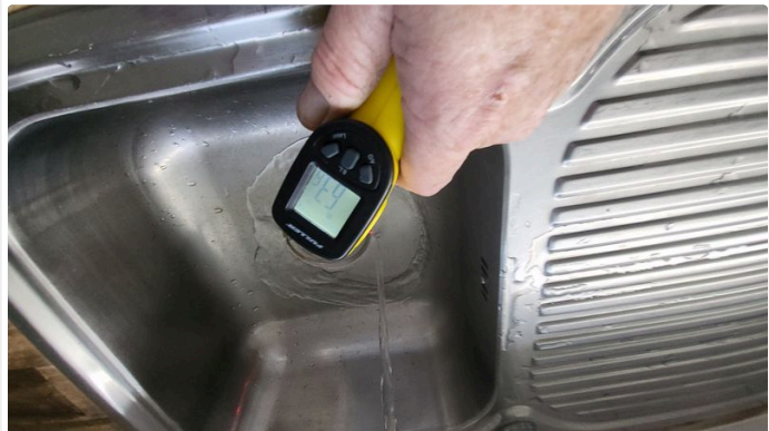
Ref #32.7 - The Hot water tested safe under 65 degrees at all outlets in the home
