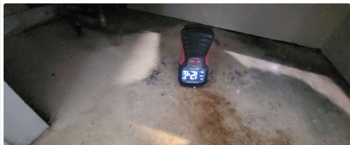
Ref # 15.5 - Tested and No Moisture was recorded at the time of the inspection
